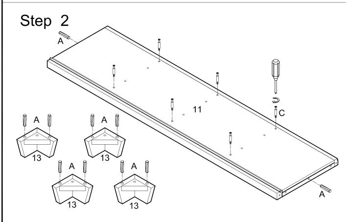
Insert dowels (A) and screw cam bolts (C) into bottom panel (11). Insert dowels (A) into legs (13).
